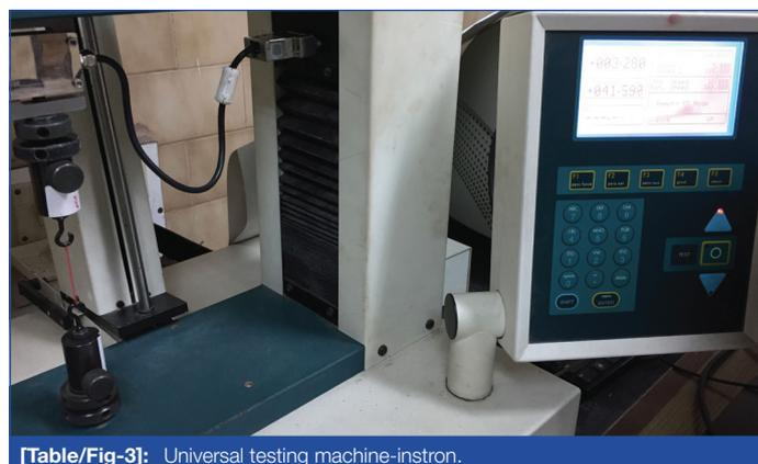
[Table/Fig-3]: Universal testing machine-instron.
