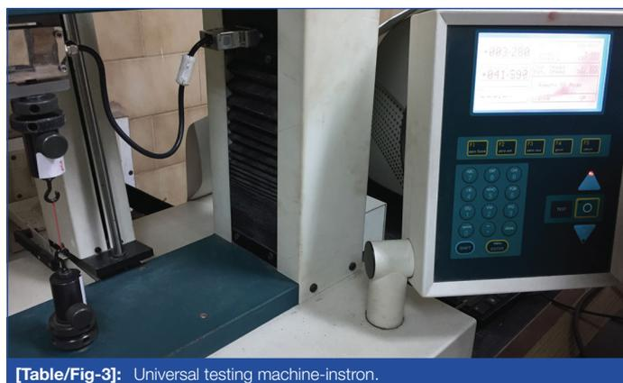
[Table/Fig-3]: Universal testing machine-instron.
