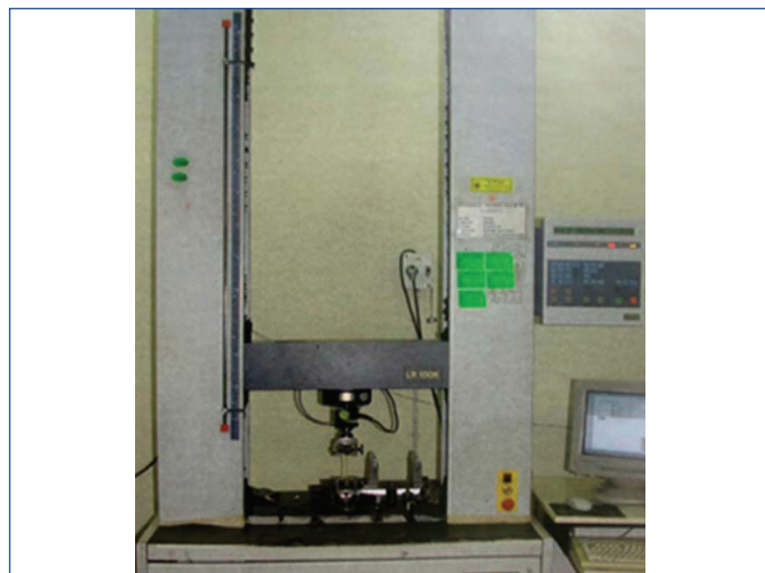
[Table/Fig-3]: Sample mounted on the LLOYD Universal testing machine.
