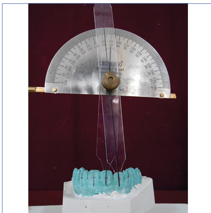
[Table/Fig-4]: Mesiodistal angulation measured on the mounted maxillary cast by the pointers on the jig.
