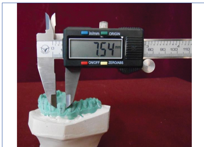
[Table/Fig-3]: Mesiodistal width of maxillary lateral incisor measured using digital vernier calliper.
