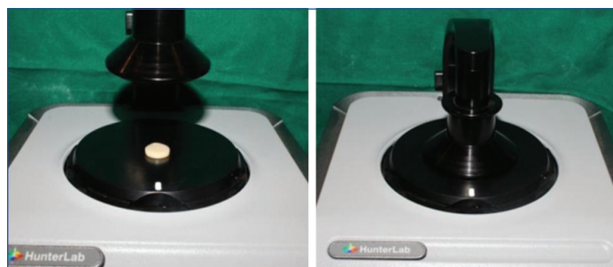
[Table/Fig-1]: Translucency measurement of ceramic sample using Agera reflectance spectrophotometer.
