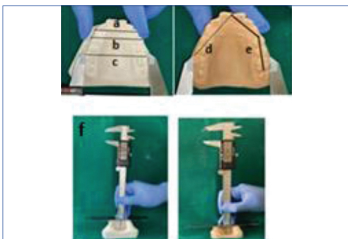
[Table/Fig-6]: Measurements using the digital caliper on a conventional stone model (Left-side) and a Rapid Prototyping (RP) (Right-side)- Arch dimensions- a: ICW; b: IPW; c: IMW; d: AL; and e: IPS; f: Palatal depth.
