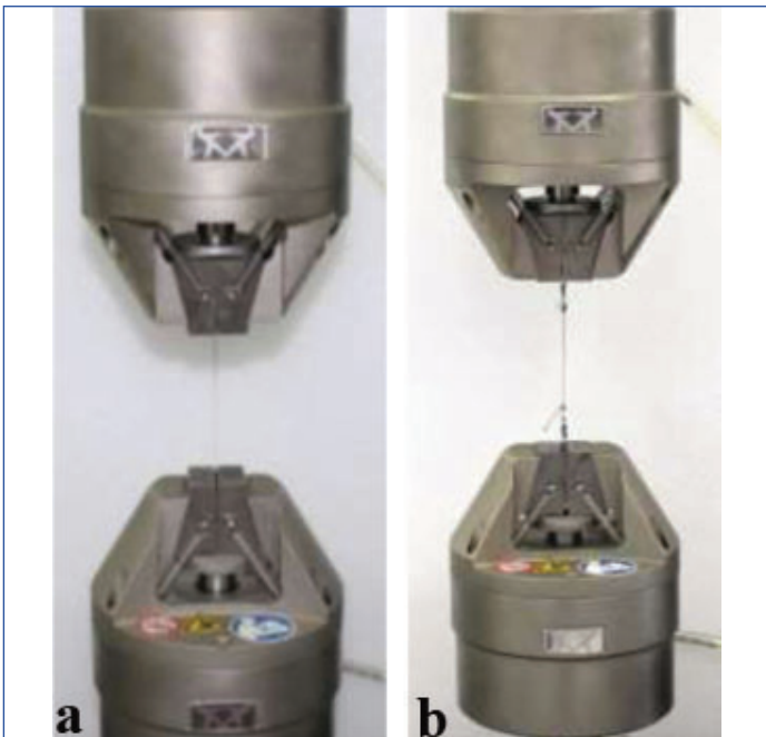
[Table/Fig-6]: (a) Straight-pull test by the Instron® method; (b) Knot-pull test by the Instron® method.
