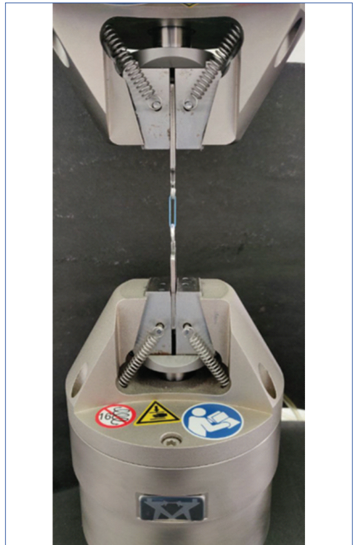
[Table/Fig-2]: The rupture strength of the elastics being tested in the Instron Universal testing machine.
