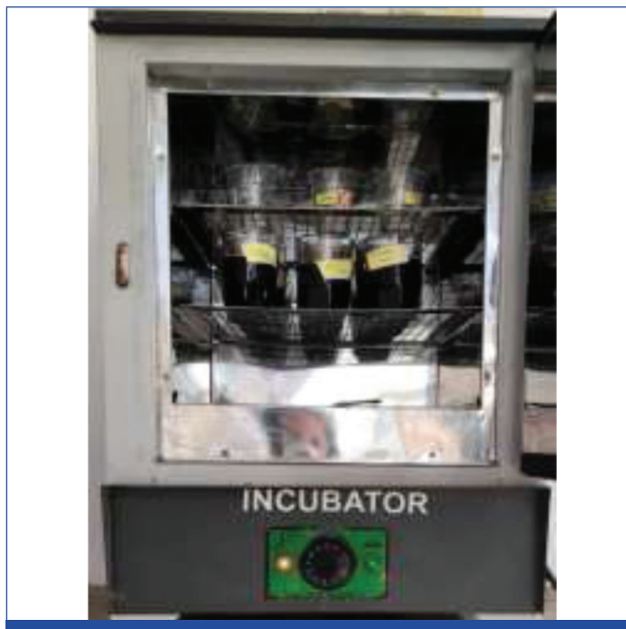
[Table/Fig-6]: The pellets were immersed in beverages and kept in an incubator at 37°C temperature for 7 days.
