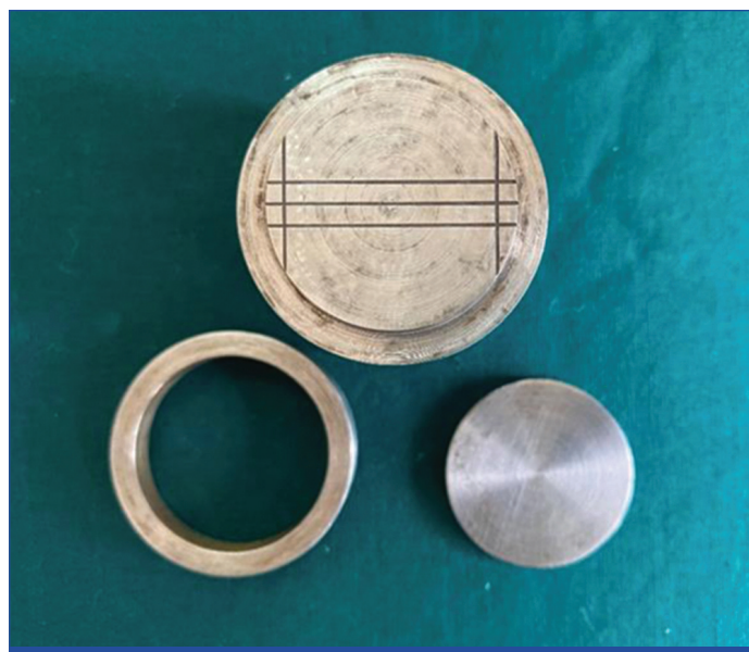
[Table/Fig-3]: Stainless steel die and ring fabricated according to ADA specification no. 19.
