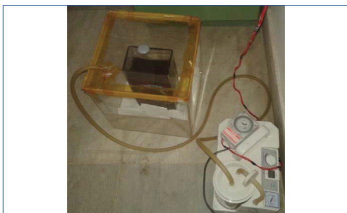
[Table/Fig-2]: Hoover chamber: impregnation with melamine.
