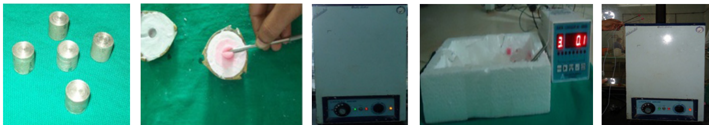
[Table/Fig-1]: Cylindrical aluminium dies for preparing the specimens to test thermal diffusivity
