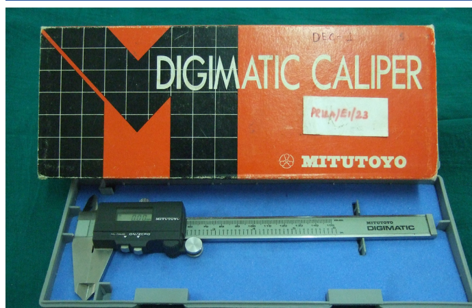
[Table/Fig-2]: Digital vernier caliper (Digimatic Caliper, Mitutoyo, Japan) 0.01mm accuracy
