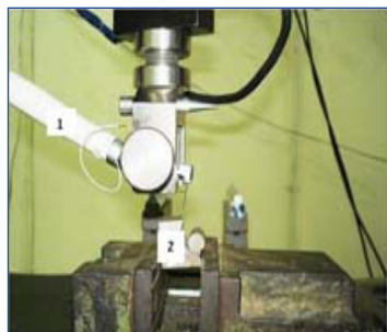
[Table/Fig-1]: Instruments used in the study. [Table/Fig-2]: Experimental set up showing (1) dental handpiece attached to the universal testing machine (2) stainless steel shaping block. [Table/Fig-3]: Shows the shaping block (1) concave radius (2) convex cylinder. [Table/Fig-4]: Notch for guiding the instruments. (Images from left to right)
