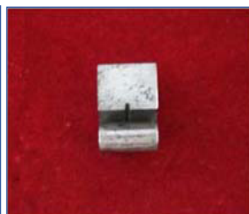
[Table/Fig-1]: Instruments used in the study. [Table/Fig-2]: Experimental set up showing (1) dental handpiece attached to the universal testing machine (2) stainless steel shaping block. [Table/Fig-3]: Shows the shaping block (1) concave radius (2) convex cylinder. [Table/Fig-4]: Notch for guiding the instruments. (Images from left to right)
