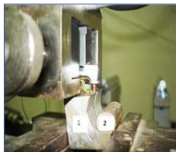
[Table/Fig-1]: Instruments used in the study. [Table/Fig-2]: Experimental set up showing (1) dental handpiece attached to the universal testing machine (2) stainless steel shaping block. [Table/Fig-3]: Shows the shaping block (1) concave radius (2) convex cylinder. [Table/Fig-4]: Notch for guiding the instruments. (Images from left to right)
