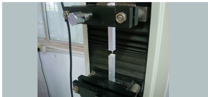
[Table/Fig-1]: Universal testing machine with mounted specimens after the tensile test
