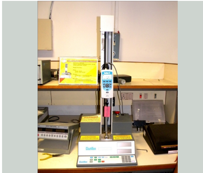
[Table/Fig-5]: Friction testing apparatus showing the ligated test wire into experimental model clamped to Instron testing machine crosshead
