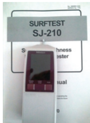
[Table/Fig-7]: Surface roughness tester
