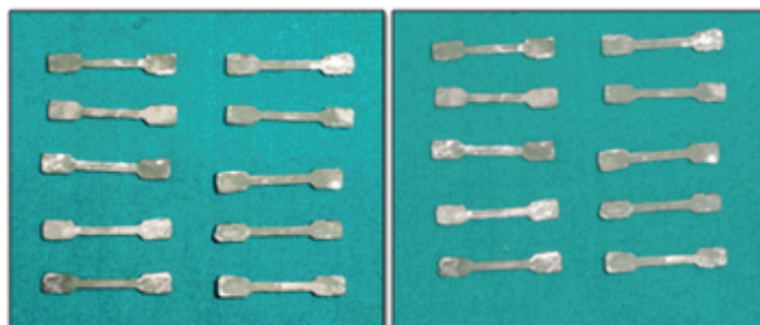
[Table/Fig-6a,b]: a) New Alloy sample & b) Recast Alloy sample
