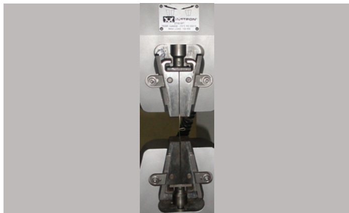
[Table/Fig-2]: Retraction loop tested in Instron Universal testing machine
