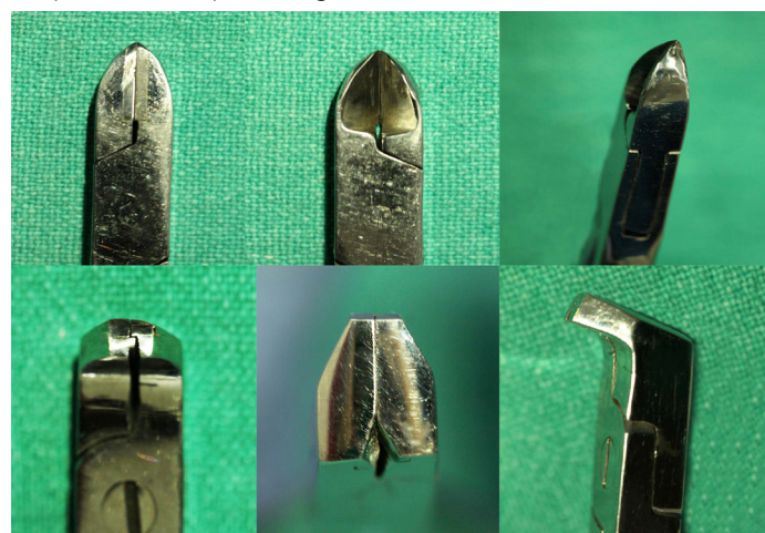
[Table/Fig-4]: Refurbished cutting edges.
