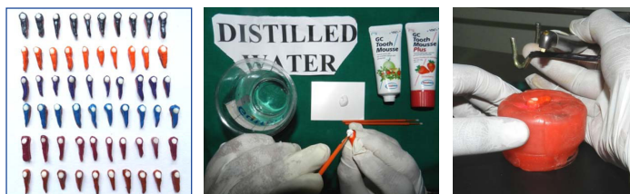
[Table/Fig-1]: Prepared enamel specimens. [Table/Fig-2]: CPP-ACP and CPP-ACFP application. [Table/Fig-3]: Er:YAG laser irradiation.
