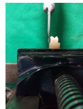
[Table/Fig-1]: Self etching primer. [Table/Fig-2]: Universal testing machine (Star Testing Systems, India. Model No. STS 248). [Table/Fig-3]: Knife-edged blade was used to apply load at the bracket adhesive interface.
