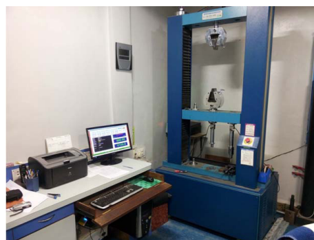
[Table/Fig-1]: Self etching primer. [Table/Fig-2]: Universal testing machine (Star Testing Systems, India. Model No. STS 248). [Table/Fig-3]: Knife-edged blade was used to apply load at the bracket adhesive interface.
