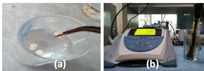
[Table/Fig-3]: (a) Immersion of pellets in 50ml deionized distilled water; (b) Measurement of fluoride release using fluoride electrode.
